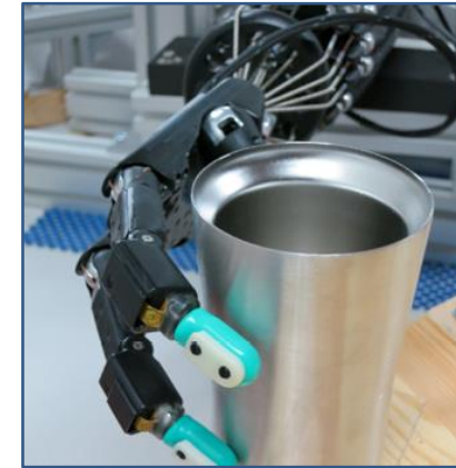
NAIST's ROS-enabled Shadow robot performing tactile object recognition.
